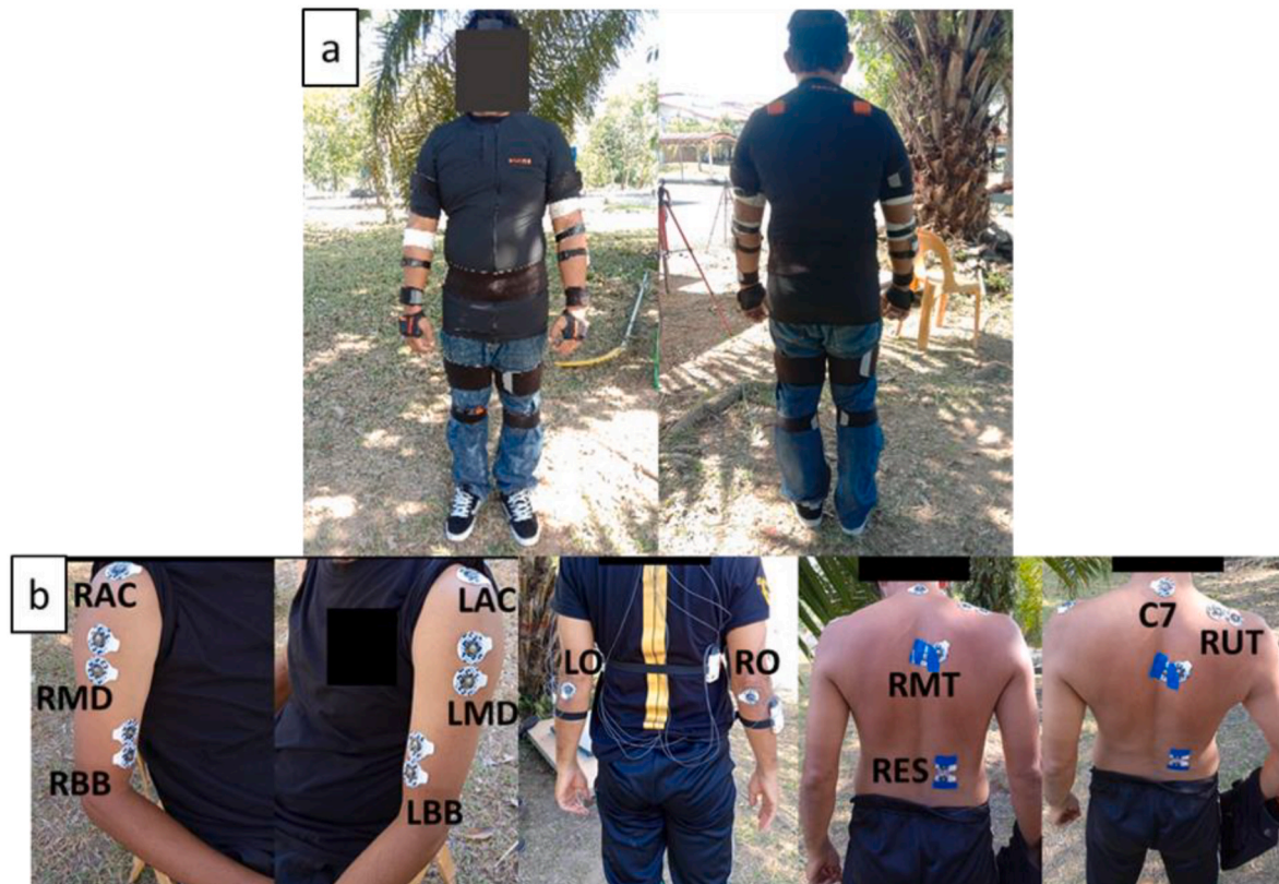
Fig. 1. (a) Xsens IMU sensors setup on the harvester in full-body configuration. (b) Surface EMG electrode placement.
