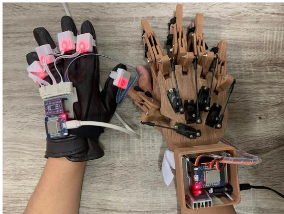
**Fig. 1.** The proposed hardware of the exoskeleton for hand rehabilitation.
