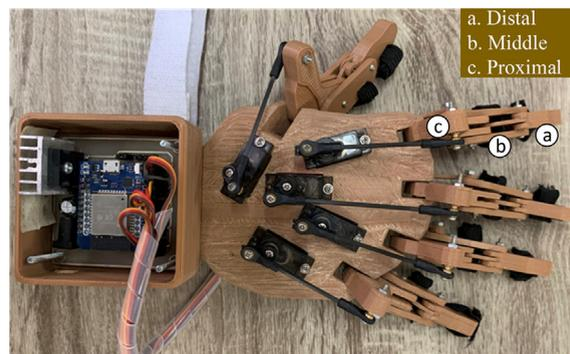
**Fig. 4.** The 3D printed of exoskeleton for hand rehabilitation which consists of 3D printing materials, servo motor, and microcontroller ESP32 Wemos D1.
