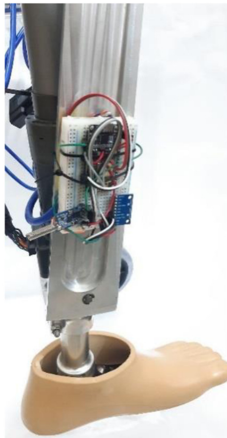
Figure 11. Smart Knee Joint with Servo Controller Circuit Attached
