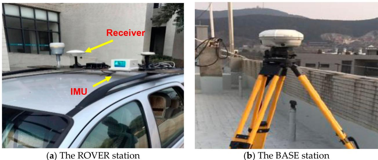
Figure 2. The basic equipment of the integrated systems.
