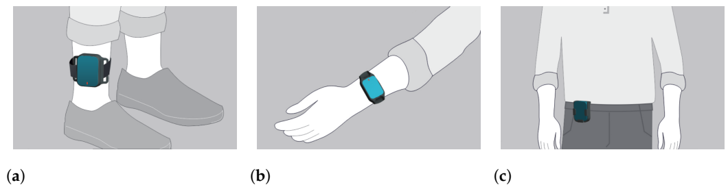
Figure 2. Placement of the wearable IMU-based monitoring devices. (a): Placement of ankle sensors. (b): Placement of wrist sensors. (c): Placement of the waist sensor.
