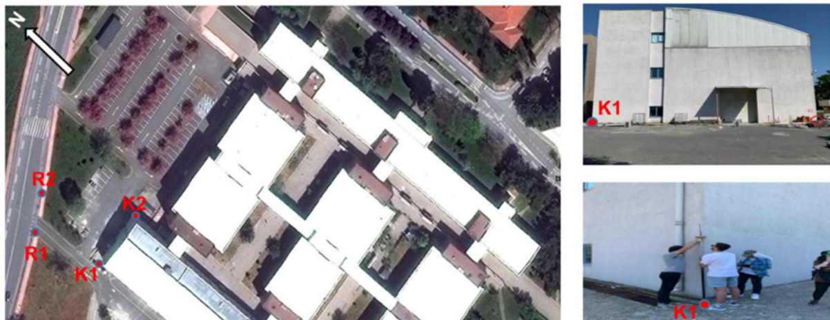
Fig. 3. The Reference Points (R1, R2) and the Corners of Building (K1 and K2 points the project area)
