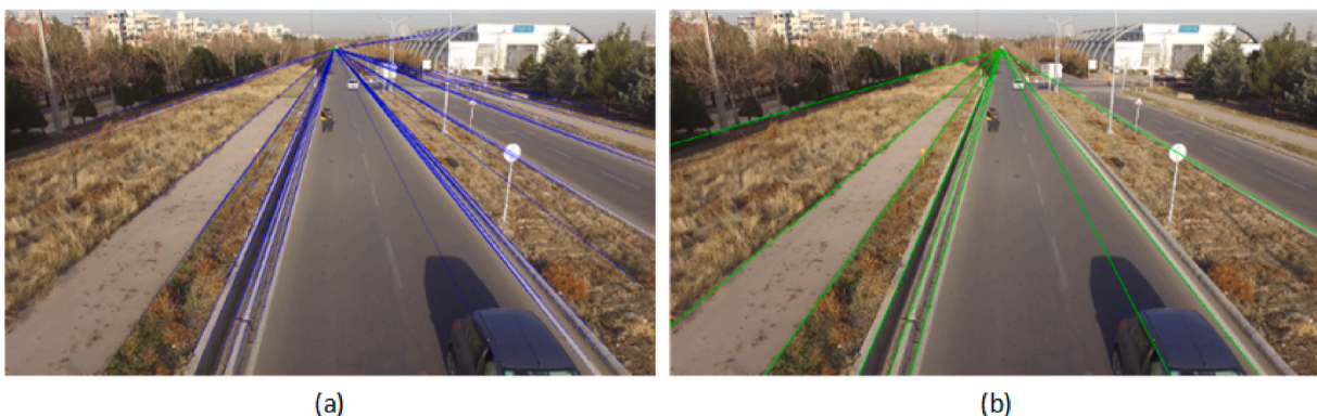
Fig. 2. Reducing line candidates. a) is before thresholding b) is after thresholding.
