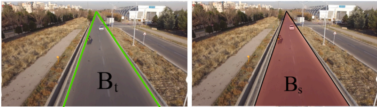
Fig. 7. This figure illustrates the road detection accuracy, B_t is the ground truth of the road area and B_s is the algorithm result of the road detected area.
