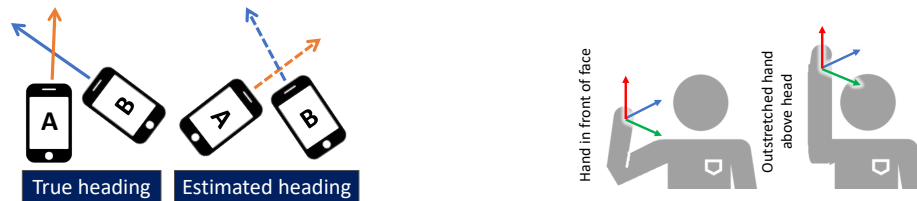
Fig. 4. (a) Wrong heading because of the magnetic field. (b) An IMU-only approach to pose estimation can lead to ambiguity.
