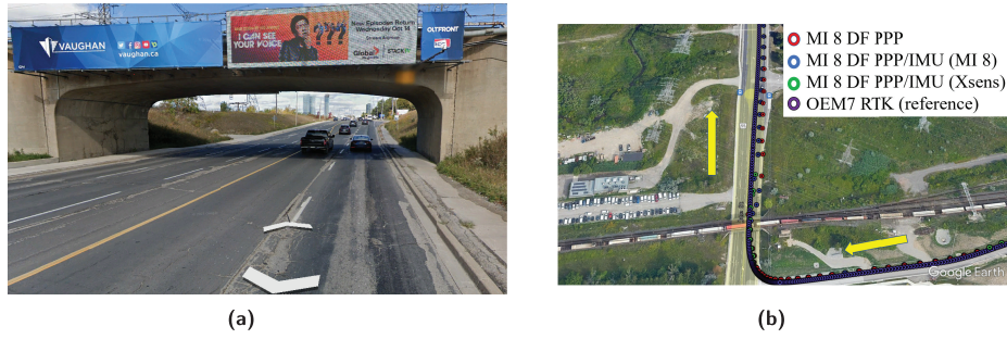
FIGURE 8 Photograph and aerial view of trajectory for Underpass A: (a) depicts a Google Earth view of Underpass A while (b) depicts Google Earth trajectories for three sensor fusion combinations.
