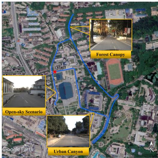
Fig. 8. The top view of the vehicle trajectory and various scenarios in the real-world experiment.
