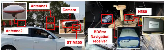
Fig. 3. The vehicle for test with equipment
