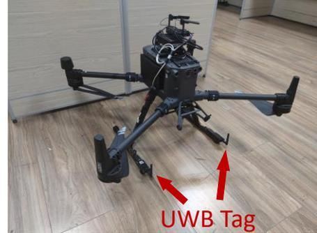
Fig. 2. DJI M300RTK and UWB tag installation position on the UAV.
