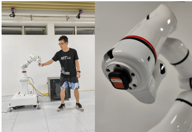
Fig. 13: The experiment scene of motion collection by a robot arm (the left panel), and the arm end with an IMU sensor (the right panel). The IMU is Xsens DOT V2 and the mechanical arm is ROKAE xMate ER3 Pro.
