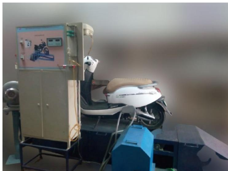
**Figure 10.** Two-Wheeler Chassis dynamometer.
