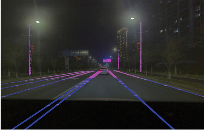
**Fig. 2.** The extracted semantic features are used to label transformed lidar points, the outlier points are dropped out.
