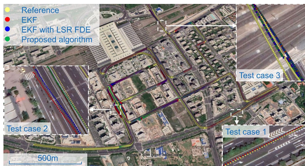
Fig. 15 Horizontal positioning results of the algorithms. Three parts of the base image are zoomed in to clearly show the horizontal positioning results in the test cases
