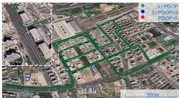
Fig. 6 GNSS PDOP value along the trajectory. The area where PDOP is higher is zoomed in as the part pointed to by an arrow shows
