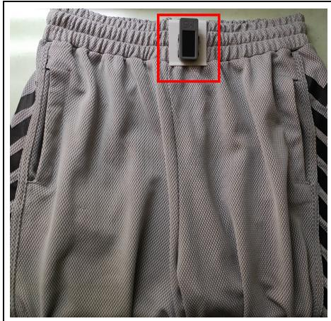
**Figure 2.** Jump meter—short connection. The red square shows the jump meter.
