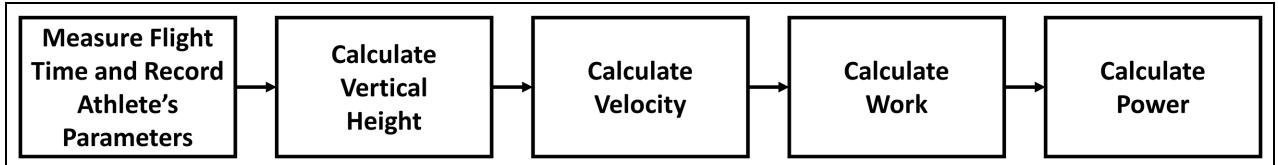
**Figure 6.** Flow chart of parameter calculations.
