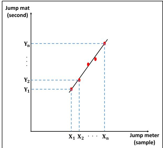
**Figure 8.** The curve fitting with the least square method to results obtained from jump meter and jump mat. In the figure, x and y represent the samples' number between two peaks in the acceleration signal, and the flight times obtained with the jump mat, respectively.
