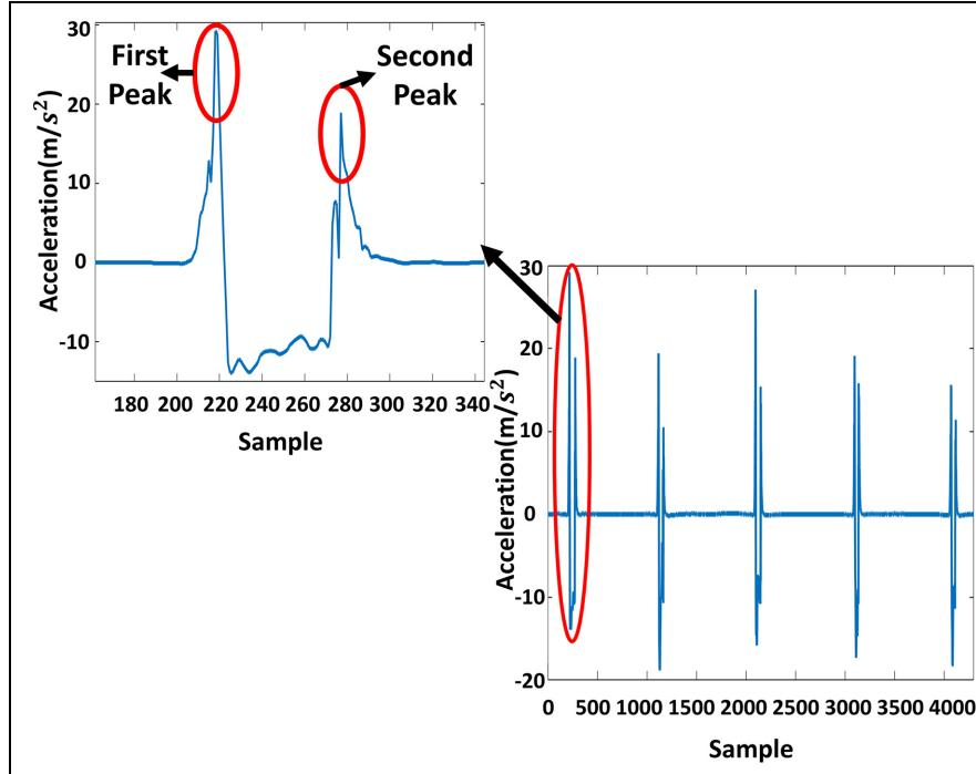
**Figure 5.** Acceleration values for five consecutive vertical jump. While the first peak occurs at the take-off, the second occurs when the person lands to the ground.
