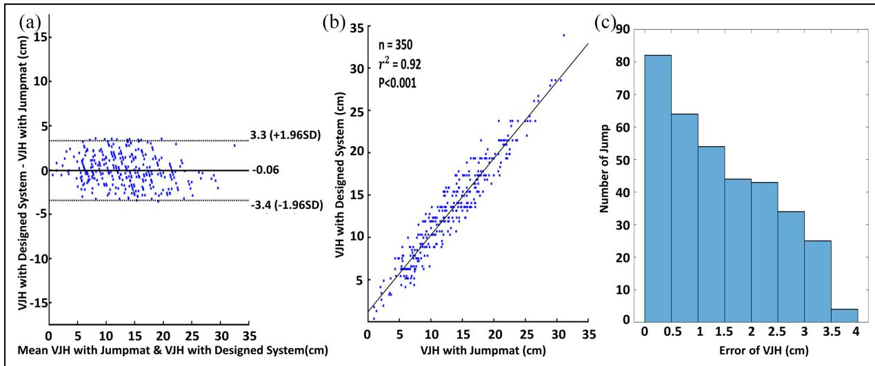
**Figure 10.** (a) Bland–Altman plots for VJH of designed system and jump mat. While the x-axis represents the mean VJH value in each jump measurement with both systems, and the y-axis represents the difference VJH value. (b) The VJH measurements with jump mat and designed system ( $n = 350$ ,  $r^2 = 0.92$ ,  $p < 0.001$ ). (c) The histogram of error values. The horizontal axis shows the ranges of error values in cm, the vertical axis shows the number of jumps in these ranges.
