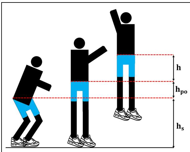
**Figure 4.** The jump movement and height parameters used at the equations. In the figure  $h$ ,  $h_s$ , and  $h_{po}$  are jump height, height of COM and vertical push-off distance, respectively.
