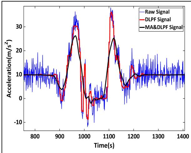
**Figure 7.** Filter effect on the acceleration signal. While the blue graph shows the raw signal, the red graph shows the signal filtered with 5 Hz DLPF, and the black graph shows the signal filtered with 5 Hz DLPF and moving average filter with 160 ms window size.
