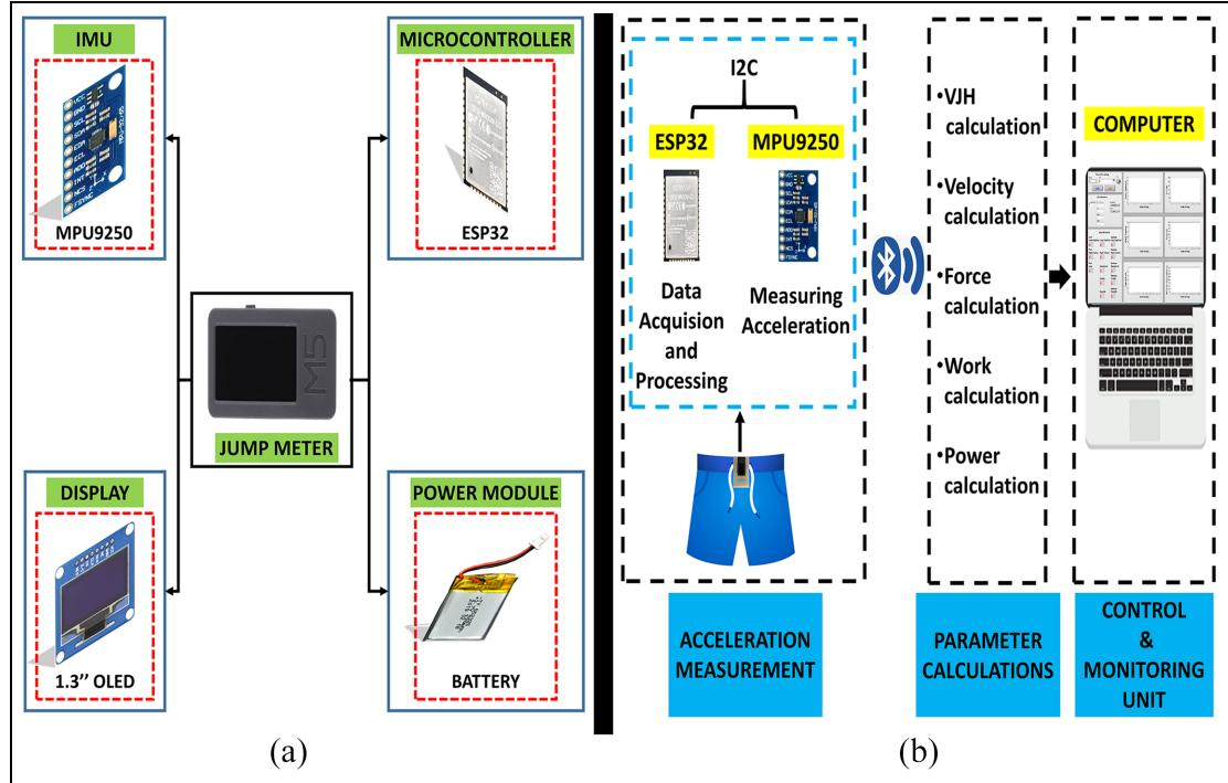
**Figure 1.** (a) The internal structure of the system. (b) Block diagram of the system.
