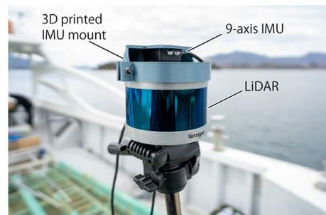
**Fig. 6** Sensor configuration of LiDAR and IMU
