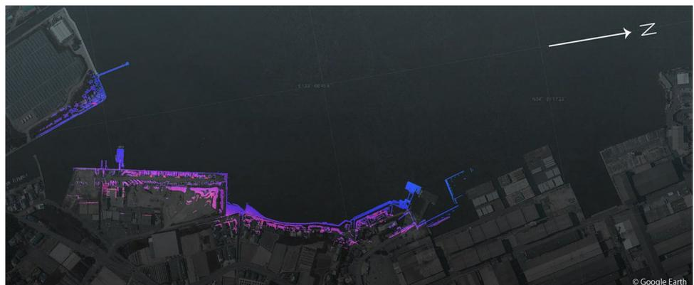
**Fig. 11** Point cloud map generated using the LIO-SAM algorithm. The background aerial photograph is referred to Google Earth
