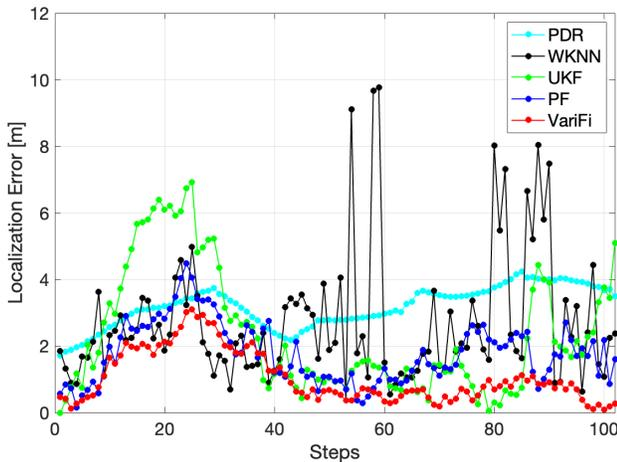
Fig. 4. Localization errors with respect to each step.
