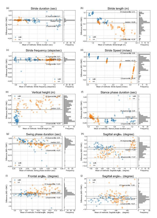
**Figure 3.** Bland–Altman plot of gait parameters from the motion sensor mounted on the shoe instep (instep-mounted) and optical motion capture (**a**) stride duration, (**b**) stride length, (**c**) stride frequency, (**d**) stride speed, (**e**) vertical height, (**f**) stance phase duration, (**g**) swing phase duration, (**h**) sagittal angle<sub>IC</sub>, (**i**) frontal angle<sub>IC</sub>, (**j**) sagittal angle<sub>TO</sub>, MS: motion sensor, OMC: optical motion capture.
