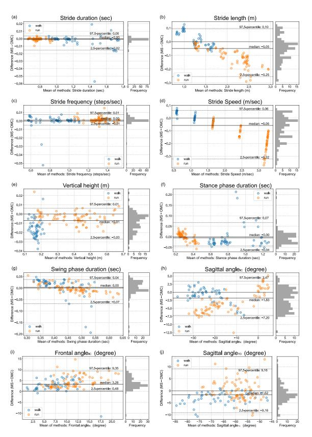
**Figure 2.** Bland–Altman plot of gait parameters from the motion sensor embedded in the shoe midsole (plantar-embedded) and optical motion capture. (**a**) stride duration, (**b**) stride length, (**c**) stride frequency, (**d**) stride speed, (**e**) vertical height, (**f**) stance phase duration, (**g**) swing phase duration, (**h**) sagittal angle<sub>IC</sub>, (**i**) frontal angle<sub>IC</sub>, (**j**) sagittal angle<sub>TO</sub>, MS: motion sensor, OMC: optical motion capture.
