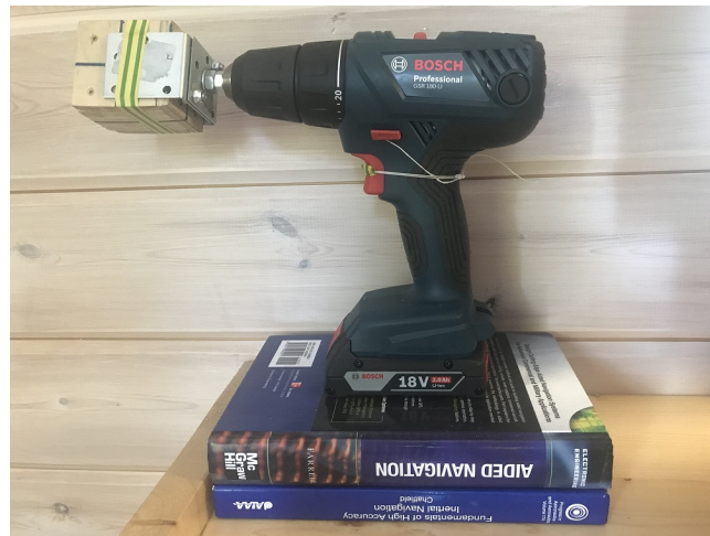
Figure 2. The IMU mounted on the shaft of a screwdriver. The IMU is inside a small wooden box which is fixed to the shaft in several positions by the adhesive tape. The trigger of the screwdriver is held by a rope in the partly pushed position to limit the angular rate of rotations (otherwise, the gyro readings are saturated). Unfortunately, for the partly pushed trigger, the low angular rates of the screwdriver we use are fairly unstable. Books on inertial navigation are of great help in the experiments.
