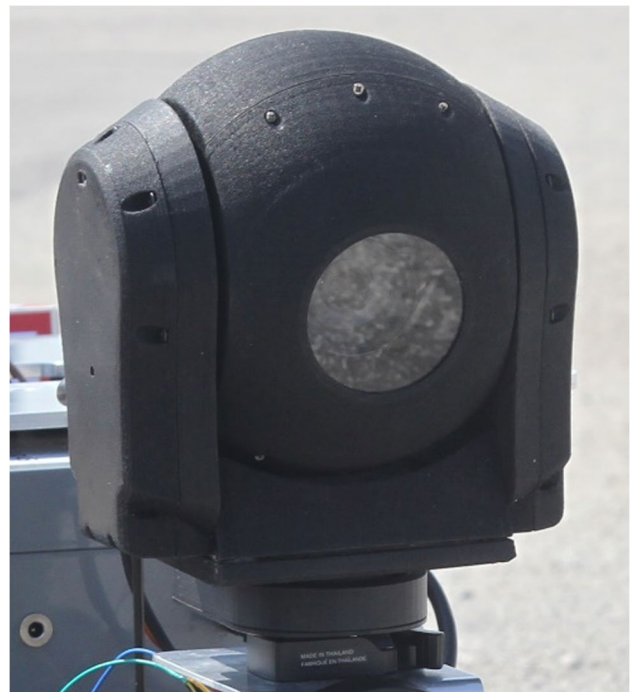
Fig. 10 TG200D three-axis gimbal
