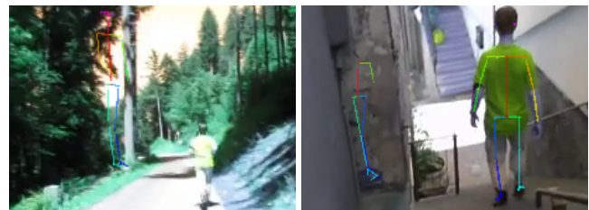
Fig. 8: Typical fail cases of OpenPose in our video data preprocessing, with downscaled video frames, background objects are wrongly recognized as human.
