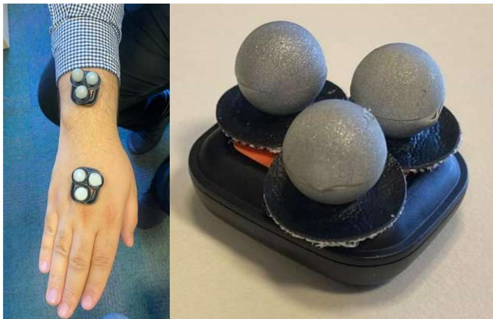
**Figure 16.** Placement of reflectors for the Vicon validation.
