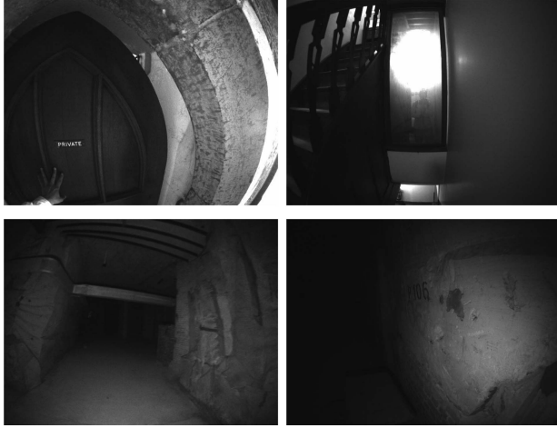
Fig. 7. Visual challenges in the NCD-Multi Dataset. Top Row: Images from NCD-Multi Stairs sequence with door opening (obscuring the cameras) shown on the left. On the right is a tight space about 1.5 m wide and a mirror. Bottom Row: Images from NCD-Multi Mine sequence with darkness and the challenge of camera being held up close to a wall.
