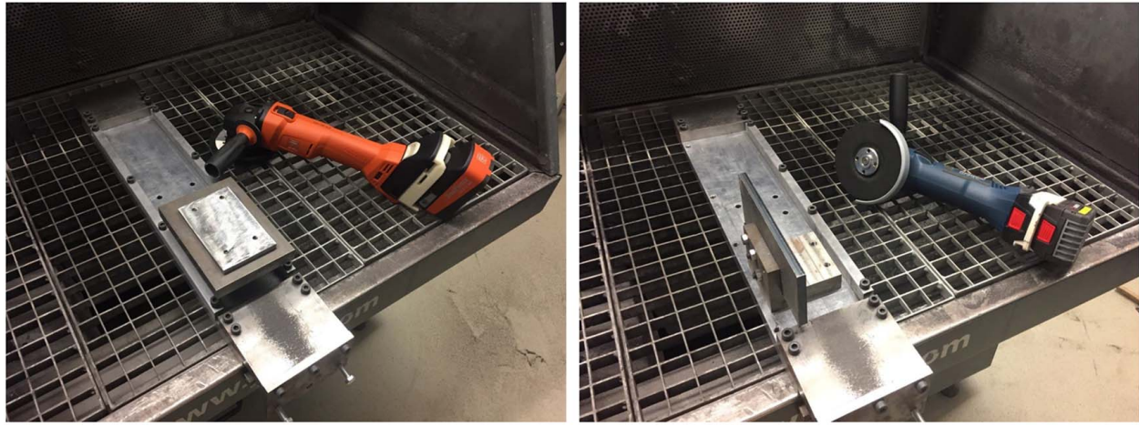
Fig. 2 Left side: CCG18 with datalogger and test setup T2 with the workpiece for grinding with an abrasive flap disc. Right side: GWS18 with datalogger and test setup T2 with the workpiece for roughing setup with abrasive roughing disc.
