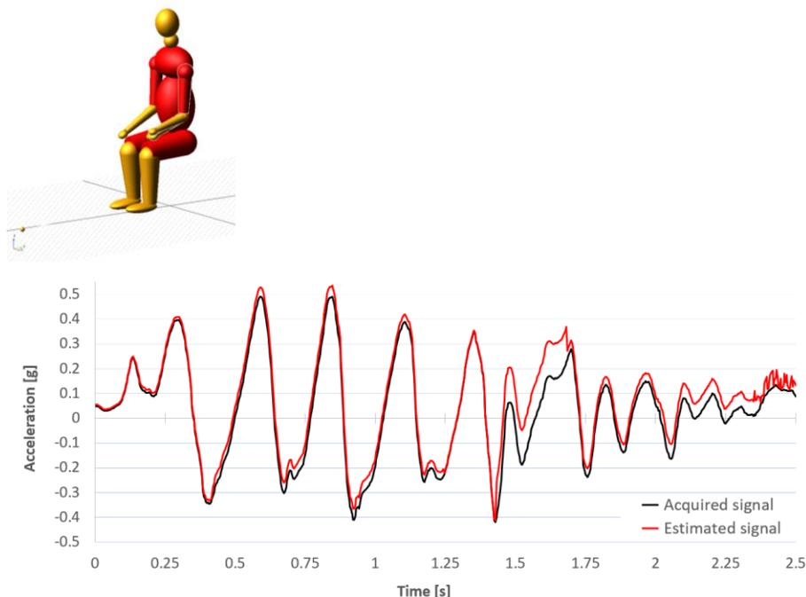
**Figure 5:** Comparison between measured and estimated acceleration signals on left hand.
