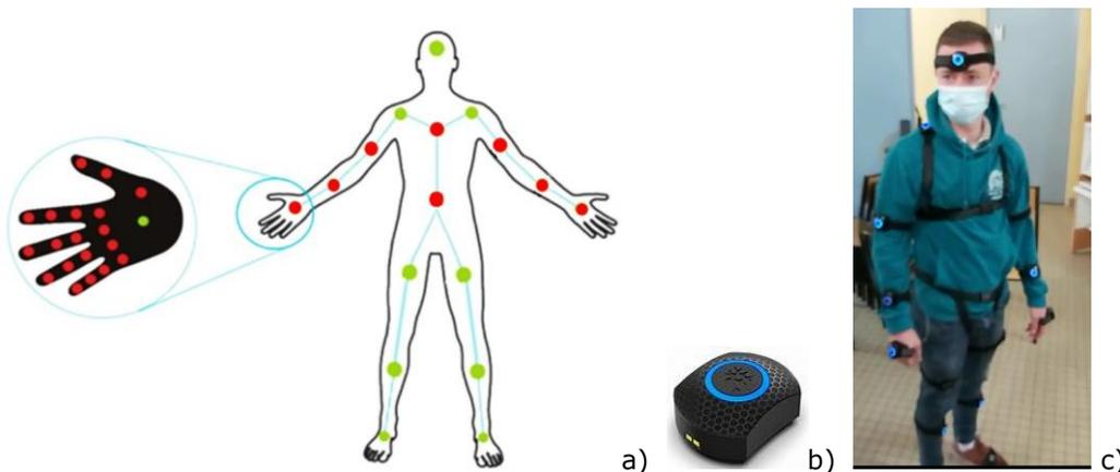
**Figure 1:** Positioning of IMU wireless sensors on the patient: (a) front (green) and rear (red) placement; (b) Perception Neuron IMU wireless sensor; (c) experimental acquisition.
