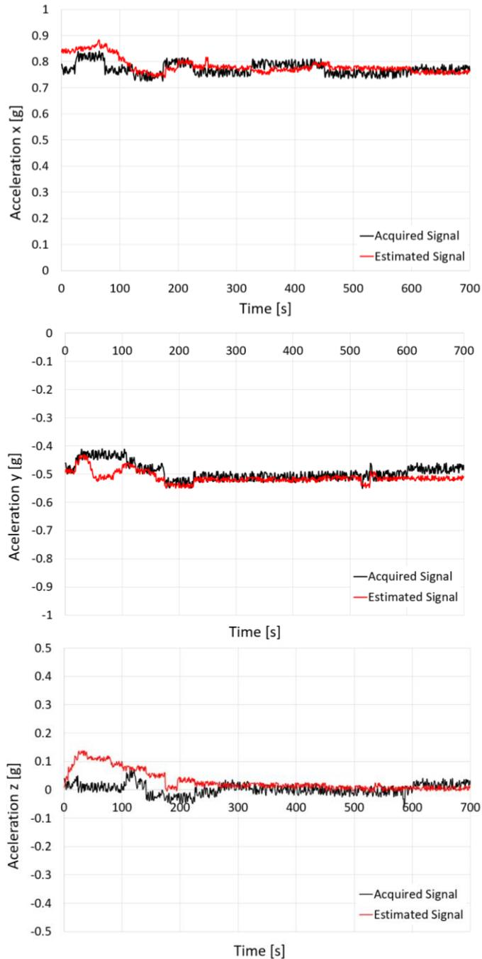
**Figure 4:** Comparison between measured and estimated acceleration signals on forearm.
